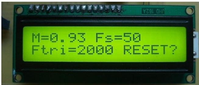
Fig. 13. LCD display showing all variables set by the user and asking for confirmation.
